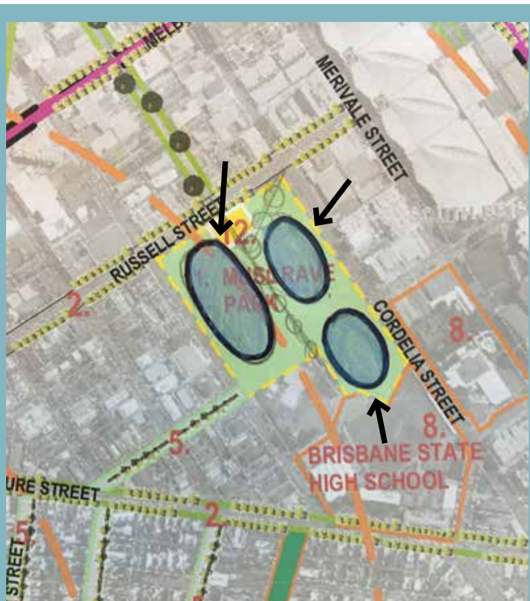
Flood plazas (shown in blue) could be created using existing large fields to harvest and filter water during extreme events.
