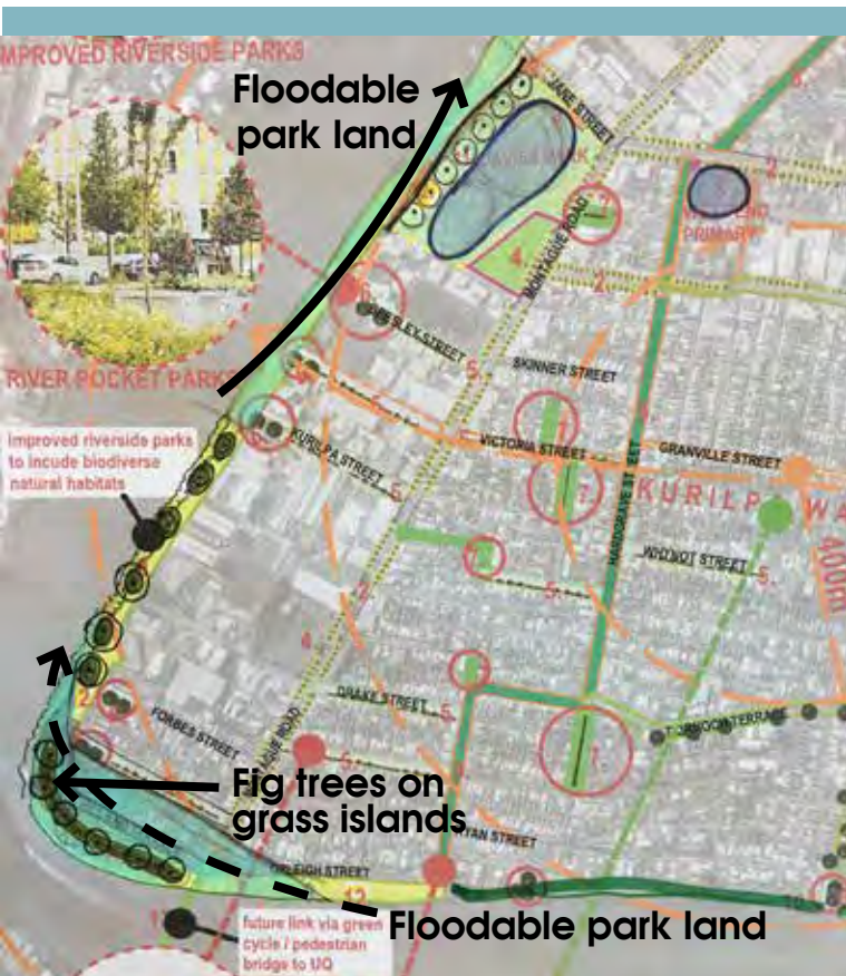
'Floodable' riverside parks could channel and slow the flow of the river during a surge.
