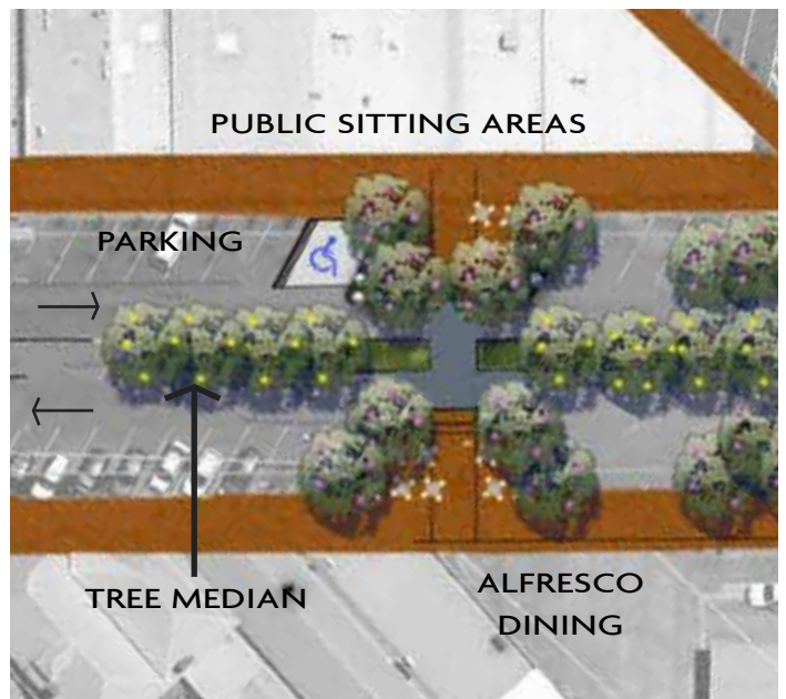
New crossings create green gateways with safe pedestrian movement and spaces for main street activation.
