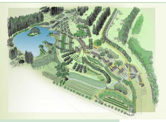
The Living Classroom is designed to redirect floodwaters into a chain of lakes and ponds connected by water holding contour swales. These areas are being revegetated to act as biological links between ecosystems. The same system of water gardens takes water from the building precinct and channels it to ponds along waterways which mimic local brooks and gullies. Water is harvested in all parts of these gardens.
